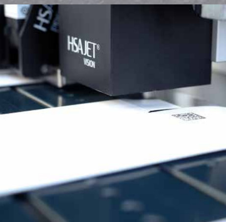
Vision Inspection Camera featuring code verification and grading.
