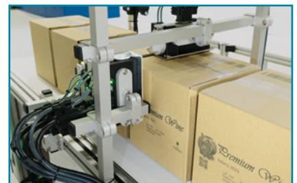
Large print swath for print of various product, branding, and shipping information directly on boxes
