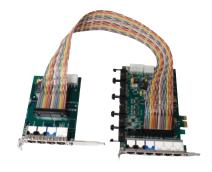
The CB6e board is based on PCI express and can control up to 4" of print height. For additional print height, a plug-board can be connected to increase the print height by an additional 4", providing a total print height of 8" via one controller board.
