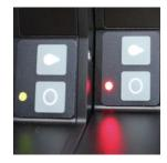
LED low ink signal and reset button on each head
