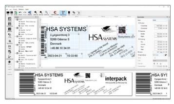
MCX UniDraw is used to design and set up print jobs for HSAJET<sup>®</sup> MCX printers. It is a user-friendly and flexible software offering all features needed to create print jobs for coding and marking applications.
